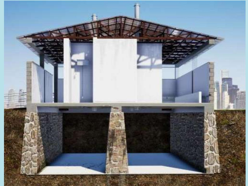
The masonry wall will have a top width of 40-50cm, and the bottom width ranges between 40-120cm depending on the soil.
