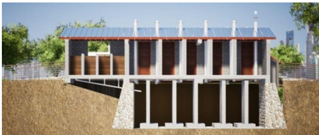
Fig 6: Composting dry pit latrine section view.
