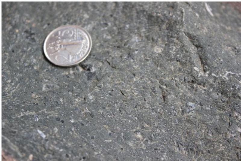
Hand-specimen: visible crystals/minerals; grey color, heavy
