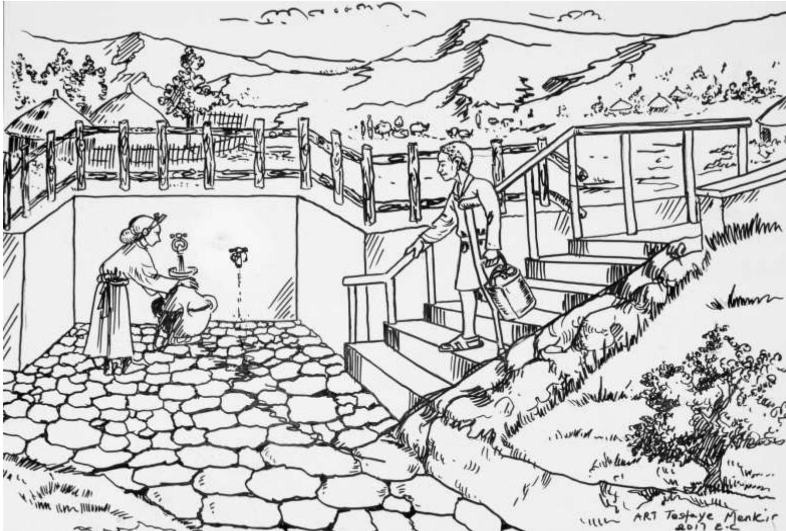
**Steps:** Where steps are needed for access, in steep terrain or when space is limited, they should be shallow and wide, and even so that all steps are the same height and depth. Depth of the step should be more than 30 cm and the height of each step no more than 16 cm.
