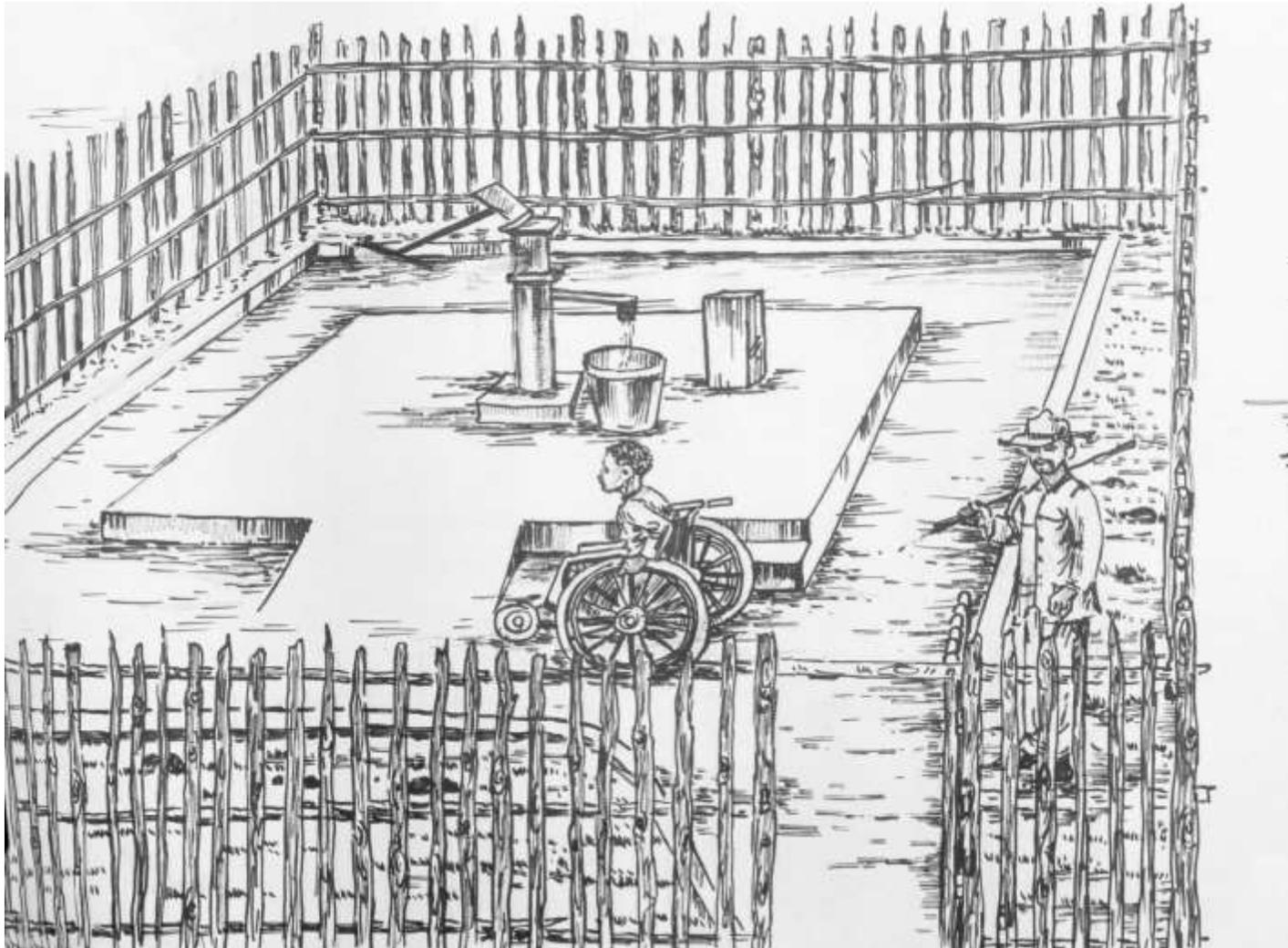
**The water supply apron** should be made accessible through a ramp and ensuring there is enough space to move around. The entrance should be wide and smooth, but not slippery. It should be ensured that if a **fence** is constructed around the facility, it should not block access to the ramp of the water point. The fence should allow easy access for all into the facility.
