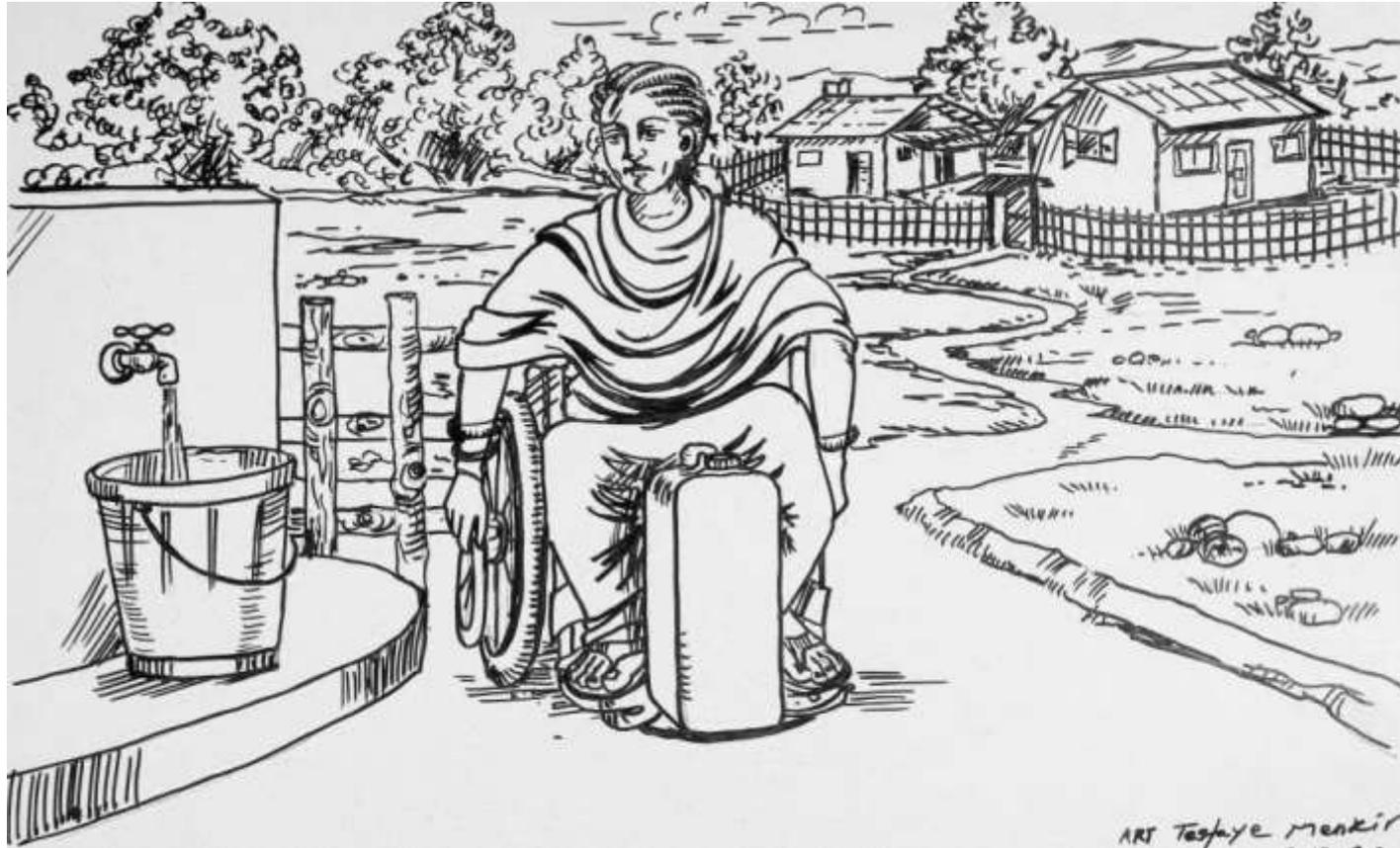
In spring protections, **taps** can be made at different heights if some cannot reach the standard height of 70 cm. For example one of the tap pipes can be bent and lowered to 50 cm.
