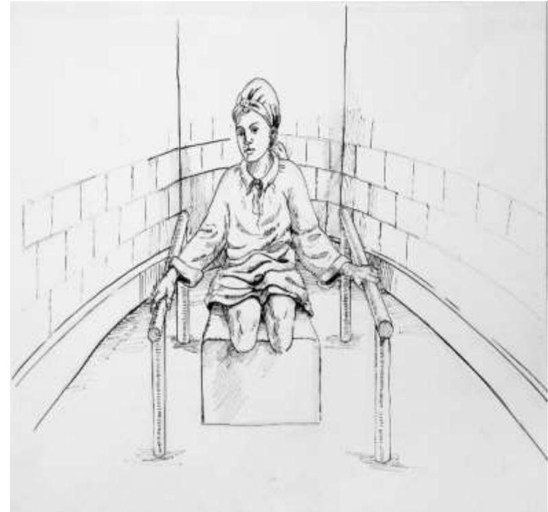
**Interior: strong handrails** (metal, wood or bamboo) can be attached to the floor or to the walls next to the toilet seat at 70-90 cm height to provide support and balance to reach the seat or squat. The position (in front or on the sides) can be assessed depending on the user's need. For visually impaired persons **tactile signs** can be important to find their way inside the toilet (e.g. mark on the wall signalling the location of the pit/ seat or a mark on the floor).
