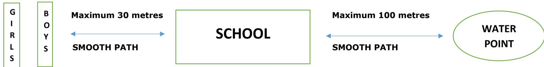
**The water supply facility** should be in the school compound or not more than 100m away from the compound with smooth and clear path. The facility or the distribution point should be made accessible for all. Taps should be placed at different heights (50 and 70 cm), close to the classrooms and the area near the taps must be made flat and ensure that it does not get muddy or slippery.
