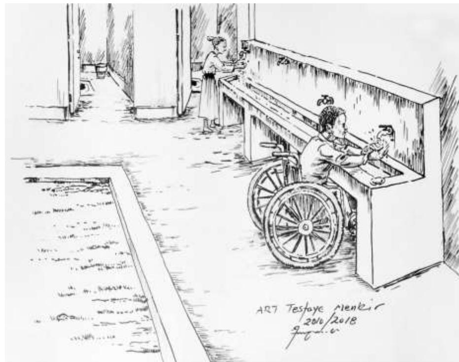
**Hand washing facilities** should be accessible for all children and staff. They should be located near to the latrines, faucets should be reachable by all and it should be ensure the ground under the facility does not get muddy or slippery.
