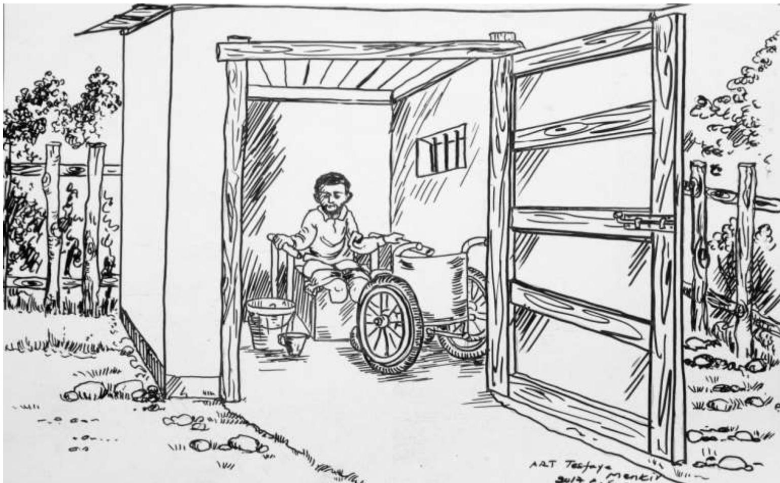
**Entrances and doors:** It is important to have a door in the toilet to ensure privacy, but the door and entrance should be wide (minimum 90 cm) and level (minimal or no difference between outside and inside). The door should be easy to open and close and can be made of locally available materials, cloth, wood or metal. The door should open to the outside. If the door opens inside it cannot be closed anymore when the wheelchair is inside.
