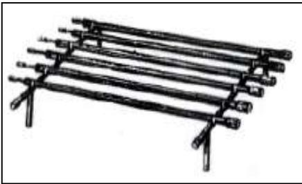
13. While removing the pipes and rods, ensure that you place these on the pipe stands. Continue doing so until the entire below-ground assembly has been removed from the tube-well
