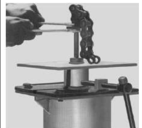
9. Place Third plate on Rod vice, take off the Chain support and remove the Chain assembly
