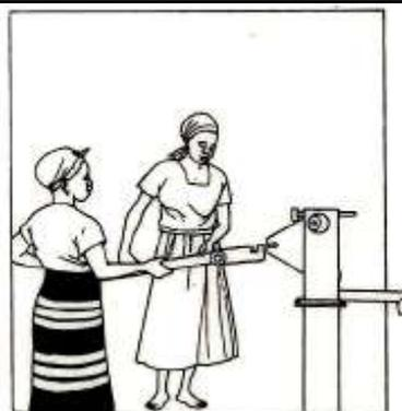
7. Raise and withdraw handle. Take care! As you remove the handle make sure the bush bearings and pin do not fall out as they may break on the floor.
