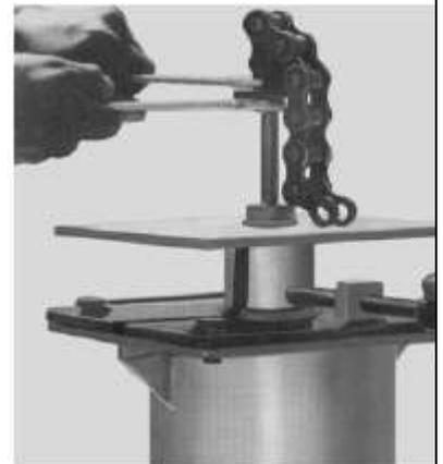
**9. Place Third plate on Rod vice, take off the Chain support and remove the Chain assembly**
