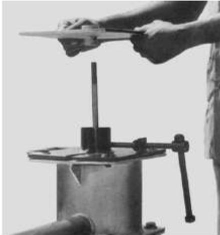
**10 Unscrew check nut and remove
