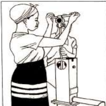
11. Pull up the hanger and first rod.
