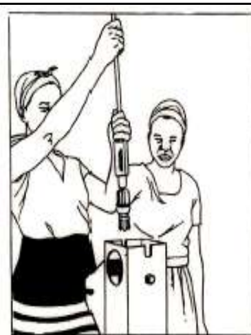
17. Remove all the rods, the fishing tool and the foot valve
