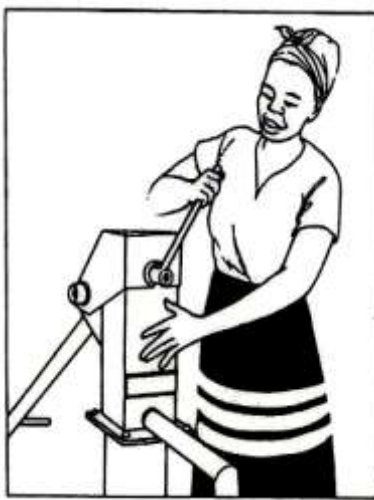
38. Tighten the cover nut
