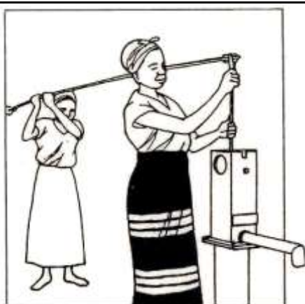
13. Disconnect and remove all rods. Remember to keep the rods in the same order. The last rod taken out should be the first rod put back..
