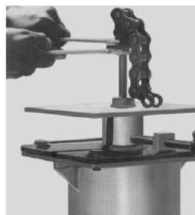
9. Place Third plate on Rod vice, take off the Chain support and remove the Chain assembly
