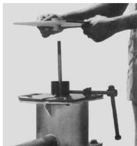
10 Unscrew check nut and remove Third plate assembly
