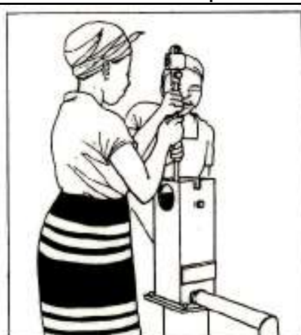
13. Disconnect and remove all rods. Remember to keep the rods in the same order. The last rod taken out should be the first rod put back..
