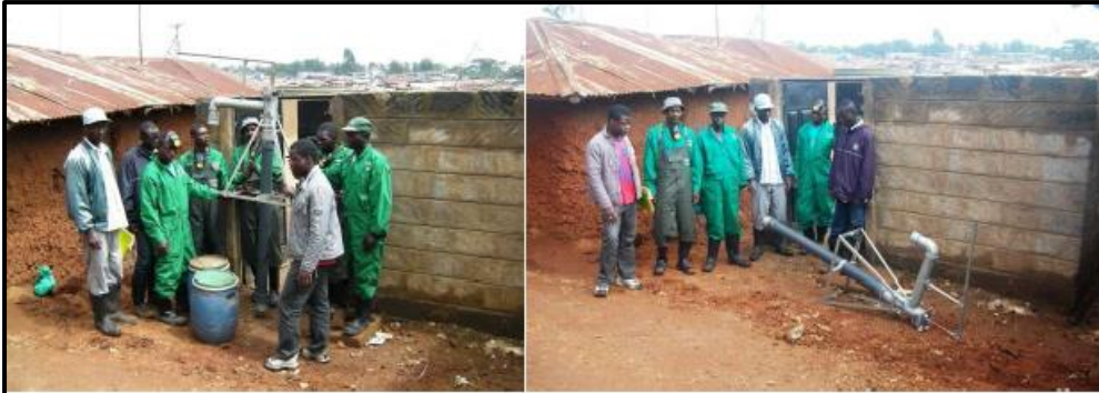
The emptiers with their short series pump at the Isha transfer station
